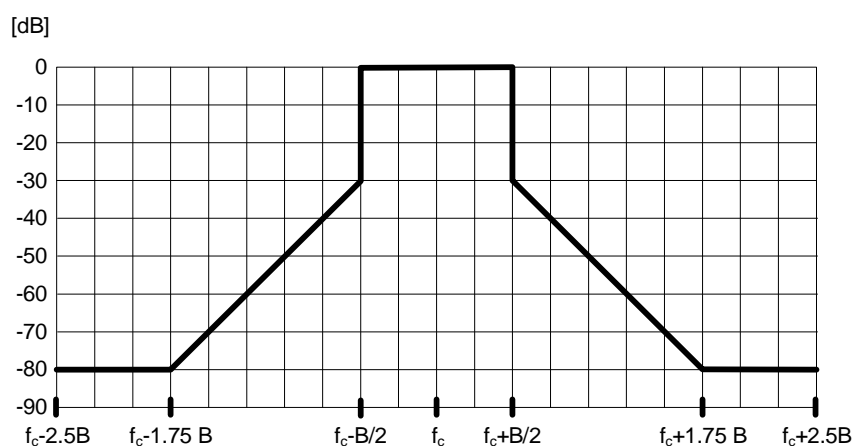
Figure 4: Transmit spectral power mask for equipment employing digital modulation, except WMAS, RBW = 1 kHz
